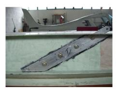
Prepare wing strut connection support cutting both edges leaving 60mm from wing strut connection outline. Clean and send the wing strut connection support section to glue to spar and glue it to the spar using structural adhesive. Let the glue dry.
