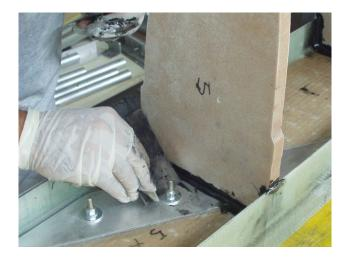
Mark nose ribs position on spar in order to ease main ribs positioning successively.
