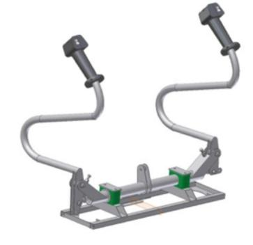
Now you can connect control stick to ailerons torsion rod through the two end rods as described in "Connecting the ailerons controls cables to the Control Stick" section and make final regulations.
