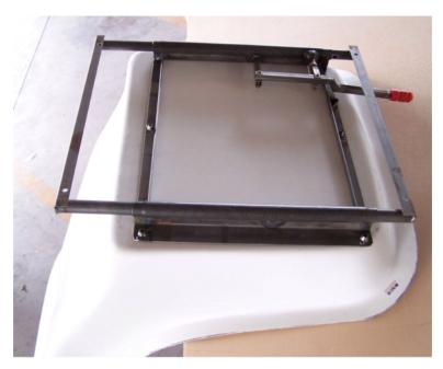
Centre seat support (or the adjustable seat support as shown in photo) on rear floor as shown below (remind the consider the rear console position) and mark position.
