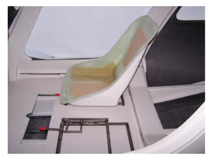
Remove seat from seat support and drill seat support fitting holes. Rivet anchor nuts to reinforcements 0260 using solid rivets 2.5. Glue with structural adhesive reinforcements 0260 to rear floor lower section in correspondence of seat support fitting holes.
