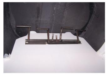
Glue with structural adhesive forward support internal reinforcements 0201 in correspondence of pedal system and control stick position, as shown in next page. Clean and send internal reinforcements before gluing.
