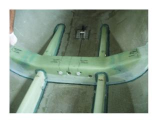
Bolt with M6 bolts and glue with structural adhesive brackets as shown below. Clean and sand before gluing.
